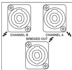
SPEAKON-type connectors are provided for the power amplifier channels „A“ and „B“. The BRIDGED OUT connector for bridged operation has a plastic coverlid preventing inadvertent misconnection.
